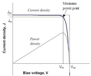
the sheet resistance is defined as  $V_m/J_m$ . The fill factor (FF) is defined as  $J_mV_m/J_{sc}V_{oc}$  and describes the squareness of the I-V curve. The efficiency  $\eta$  is defined as the ration of power density delivered per unit incident light power density:
