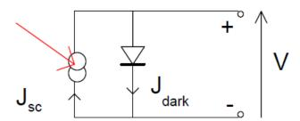
Fig. 1.7. Equivalent circuit of ideal solar cell.
