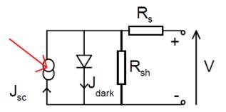
Fig. 1.10. Equivalent circuit including series and shunt resistances.
