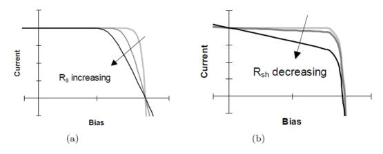
The contact resistance must be small. This appears in series. Sometimes there is leakage current through the cell and <u>around the edges of the cell</u>. This is equivalent to a parallel resistance. This must be large for good performance.
