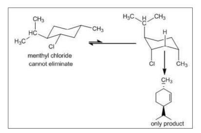
**Scheme 6.** Elimination of menthyl chloride under alkaline condition.
