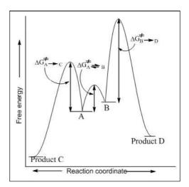
**Figure 1.** Free energy profile diagram for Case I.
