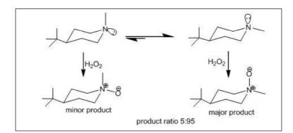
**Scheme 7.** Oxidation of 4-*t*-butyl-*N*-methylpiperidine.
