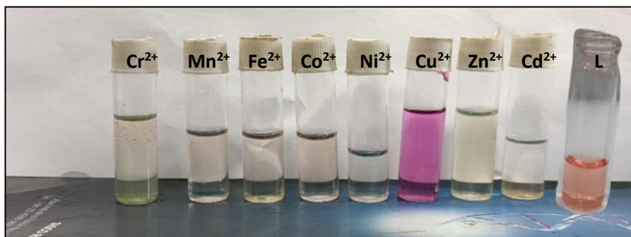
Visible colour change of chemosensor in presence of various metal ions
