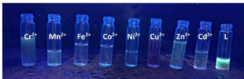
Fig b: Fluorescence check chemosensor- L in presence of various metal ions under UV lamp
