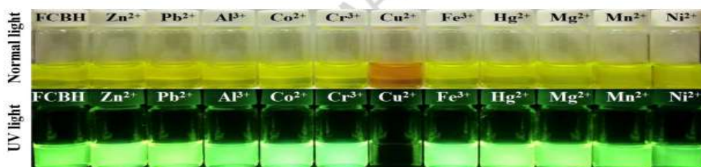
Fig. 1. Naked-eye and fluorescence images of FCBH (20 \mu\text{M} , DMSO/water, 1:1) upon addition of various metal ions (1 equiv.).
