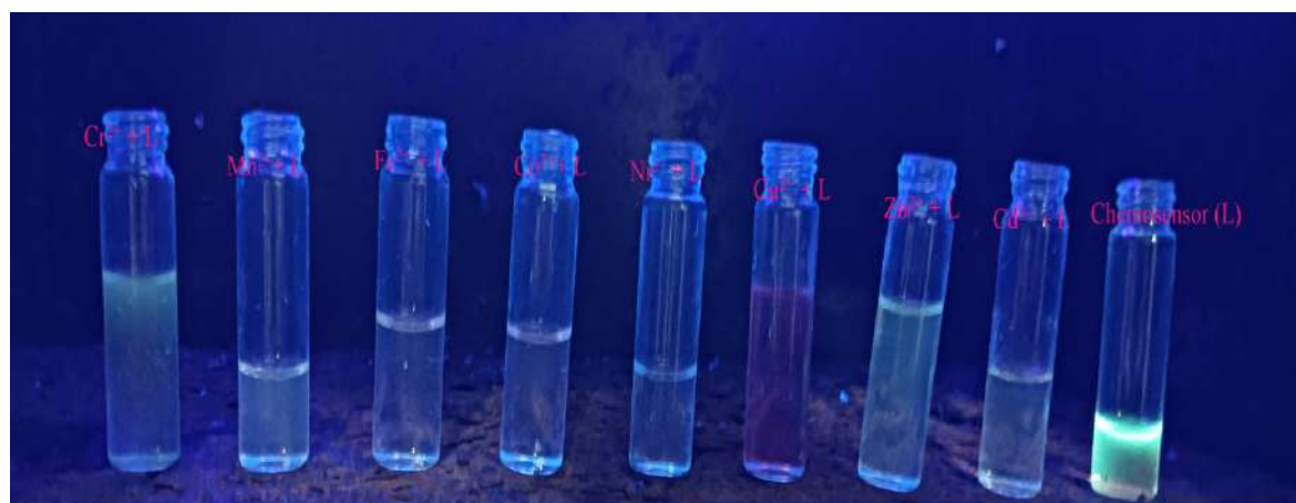
Fluoremetric change of metal cations in stock solutions and Chemosensor (L) in presence of Fluorescence light.
