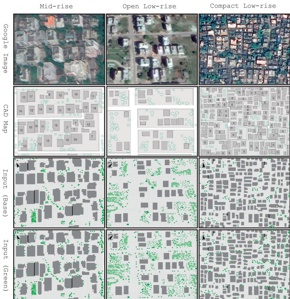
Fig. 2. The view of three model areas (Mid-rise, Open low-rise and Compact low-rise at abscissa direction and Google image, CAD map, input file of Base model, and input file of Green model at ordinate direction) for ENVI-met simulations with pink dots of receptor on streets over the KMA region.
